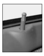
To lock the door from the inside, push down on the manual lock rod located on the door. To unlock it, pull up on the manual lock rod.
